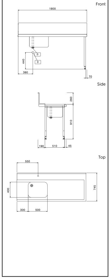
Handling System for Hood type Pre-wash Table with Bowl Right to Left, 1800mm
